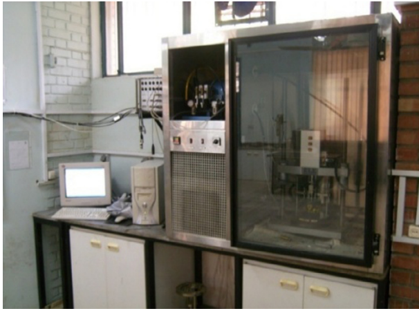
Fig. 5. UTM-5 apparatus equipped with temperature control chamber.
